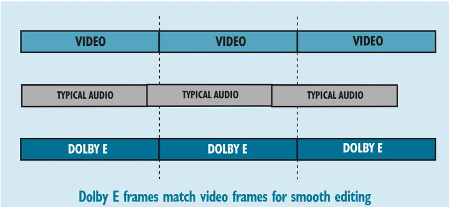
Dolby E adds one frame of delay during encoding and one frame during decoding, and requires a "color-black" reference signal to keep audio and video frame rates locked.
